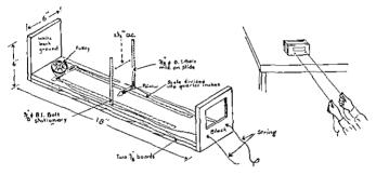
FIGURE 34.- Equipment for depth perception test.
